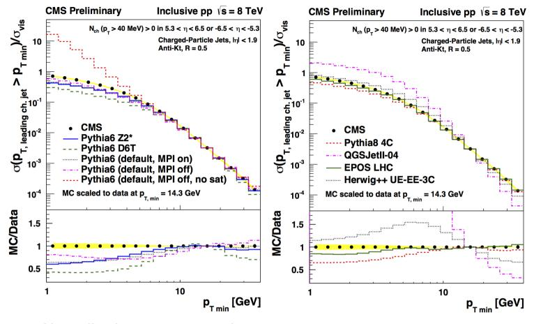
Normalized cross-sections for events with a central leading charged particle with  $p_{T} > p_{T,min}$  as a function  $p_{T,min}$ .
