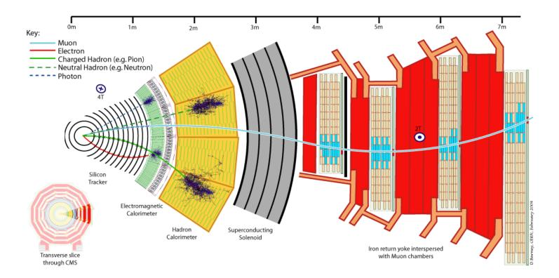
Tracking: |η|<2.5 Central Calorimetry: |η|<3 Forward Calorimetry: 3<|η|<5
