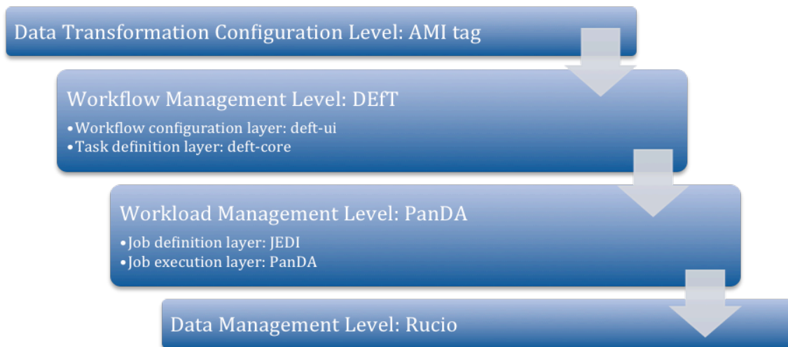
Figure 5. Multi-level architecture of the ATLAS Big Data processing infrastructure for Run 2.
