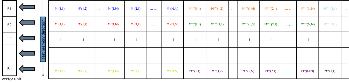
Figure 4. Memory layout for the new matrix library MATRIPLEX. The layout is optimized for our problem, which consists of matrix manipulations of low-dimensional matrices. The memory layout is matrix-major. In the Figure, the matrix dimension is N \times N and the vector unit size is n .
