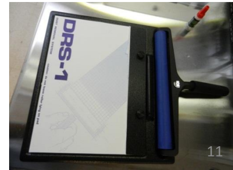
Tacky roller → dust removal
