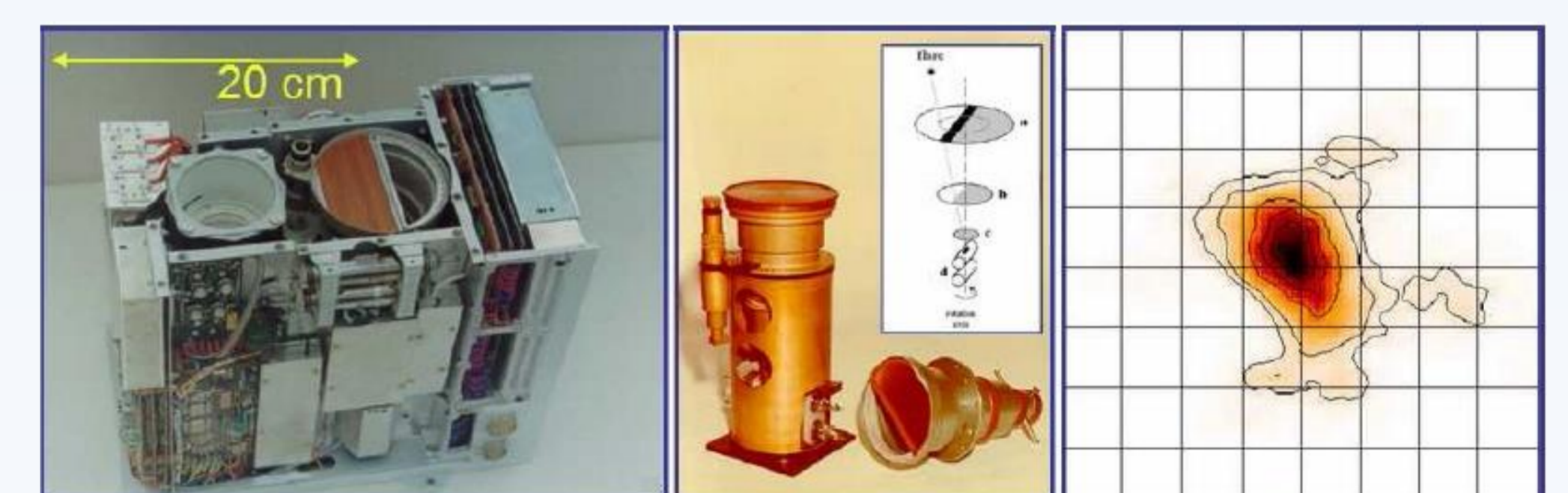
Figure 3: Left: RF15-I soft X-ray Photometer-Imager flown on INTERBALL-Tail mission. Center: Imager assembly of RF15-I, Right image obtained from RF15-I (grid is 50x50 arcsec).
