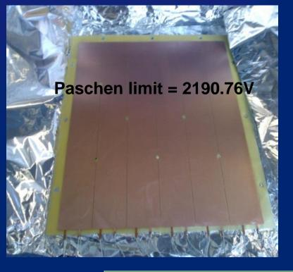
The Paschen limit is used to check the breakdown voltage of the THGEM as received from the company and after the treatment (see table). For this piece the treatment was repeated twice. The 6 different sectors could reach breakdown voltages near the expected limit.
