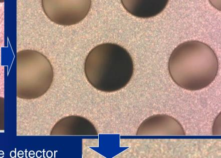
Smooth hole edges improve the detector field uniformity reducing the possibility of having high values of the E field due to sharp hole edges. Larger AV can then be applied and consequently larger gain can be achieved.
