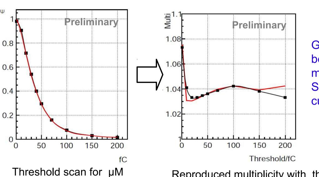
Good correspondence between the measured multiplicity (black curve) & Simulation+Digitizer (red curve)
