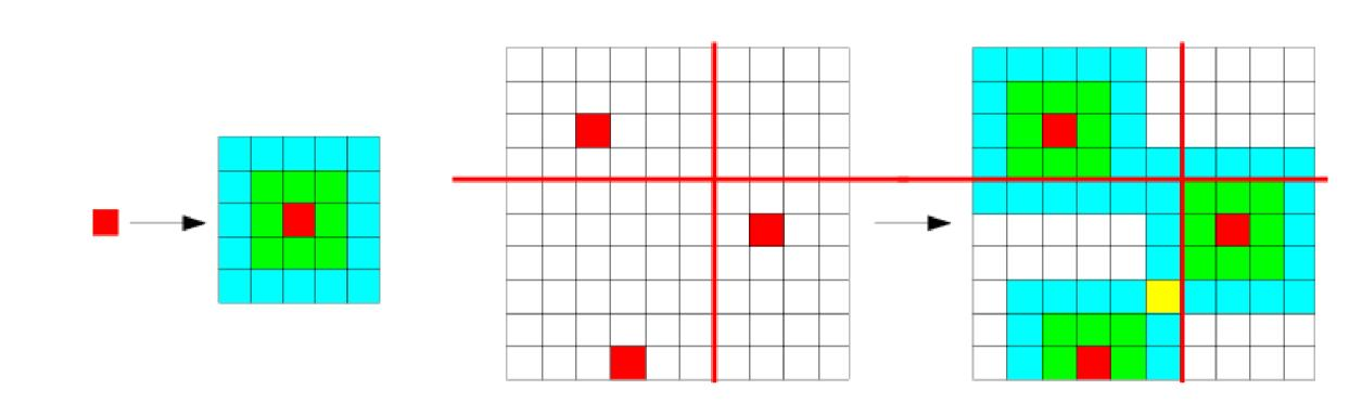
Simulated hit  $\rightarrow$  charge spatial table  $\rightarrow$  charge accumulation  $\rightarrow$  apply the threshold
