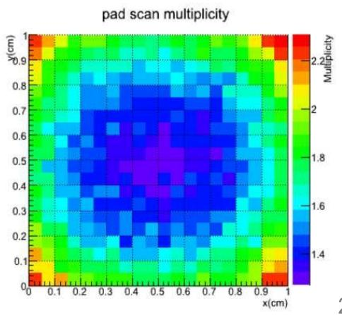
The fraction of the charge induced on each pad is inferred from the 2D integration of a known profile and the precise position of the GEANT4 hit.
