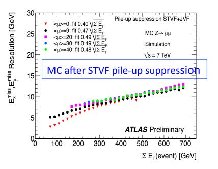
•  $E_{x,y}^{\text{miss}}$  resolution closer to the resolution in after pile-up suppression with STVF
