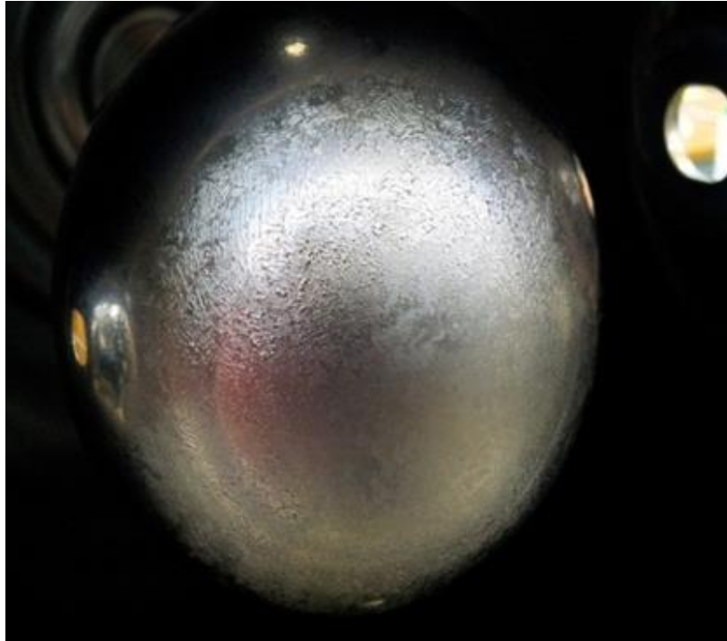
Central electrode: 20 mm diameter, at earth potential
