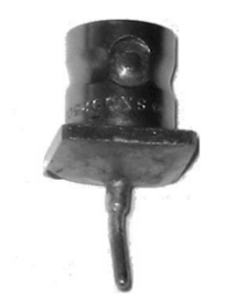
BNC Shunt for current injection (for Zt of Coaxial cable assessment)
