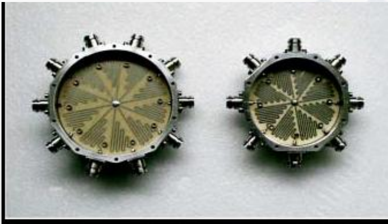
SOLEIL stripline splitters, using \lambda/4 transformers
