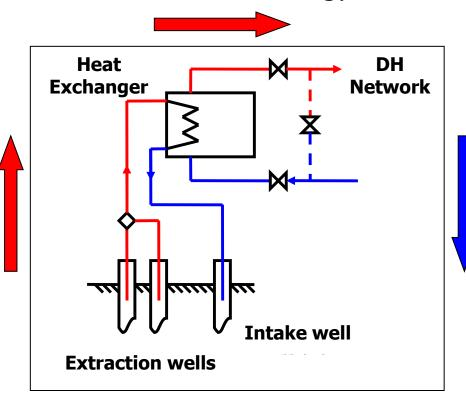
The fluid is reintroduced in the ground in order to ensure the geotechnical stability.
