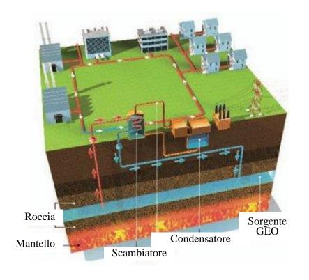
Exploitation of the geothermal resource as a primary source for a D.H. system
