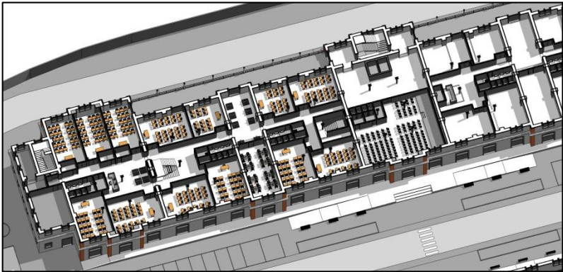
First floor - 3D section
