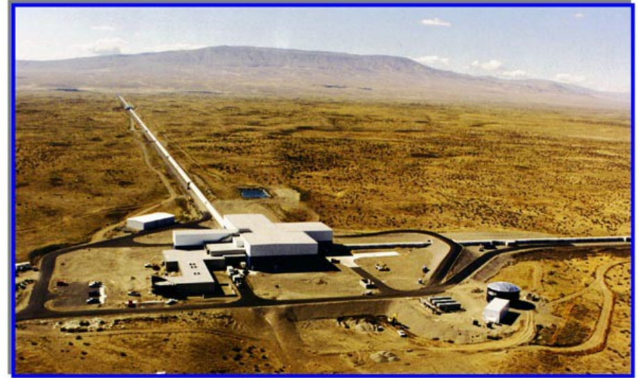
LIGO: Two interferometers in the US with 4 km, one with 2 km arm length
