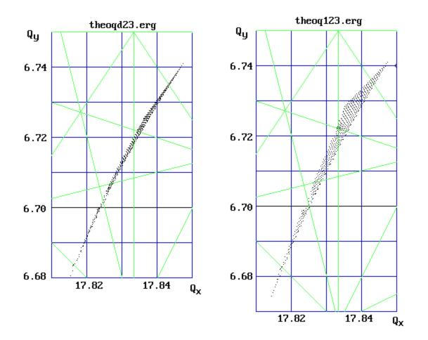
Modification of the calculated frequency map if the dipole fringe field is included (right).
