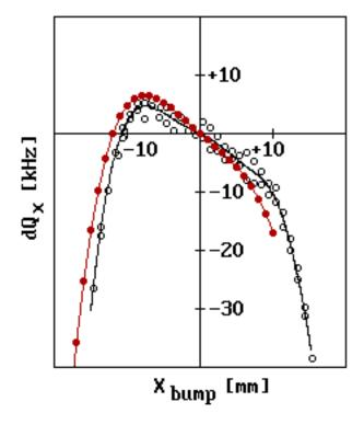
Horizontal tune as a function of a horizontal closed orbit bump. Theoretical prediction is shown in red and experimental result in black. Harmonic sextupole magnets were turned off and the chromaticity was set to zero during the experiment.
