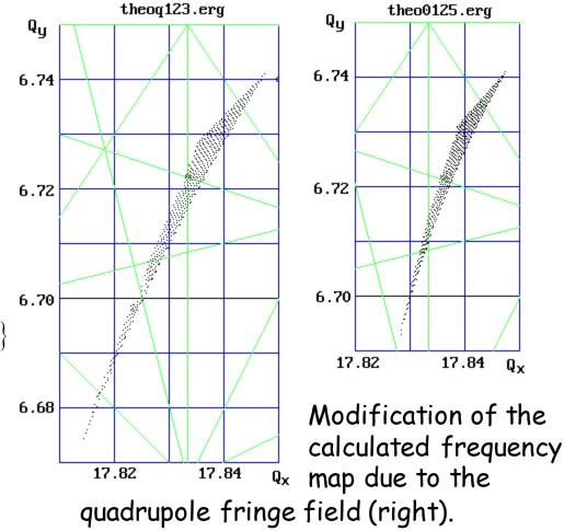
Quadrupole fringe field important as soon as amplitude dependent tune shifts are small
