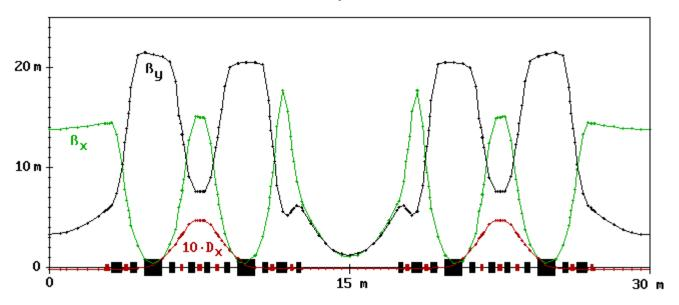
Optics functions of 1/8 of the storage ring as a result of a response matrix analysis
