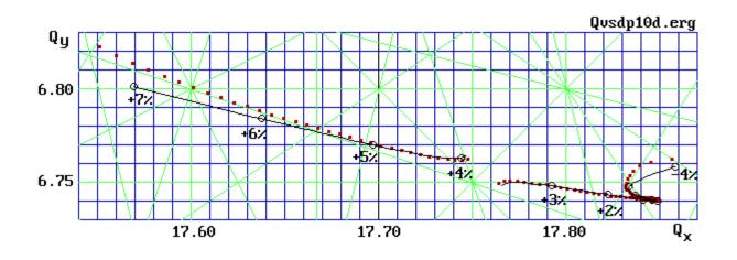
Momentum dependent tune shift calculated taking dipole and quadrupole fringe fields into account. Measurement is shown in red.
