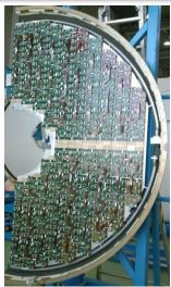
Various VLSI chips for X-ray detection
