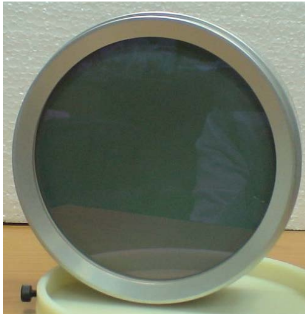
120 mm diam deformable mirror for 100 TW beamline
