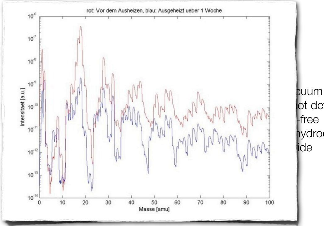
vacuum is not defined by pressure: example of mass spectrum before and after baking the a test chamber
