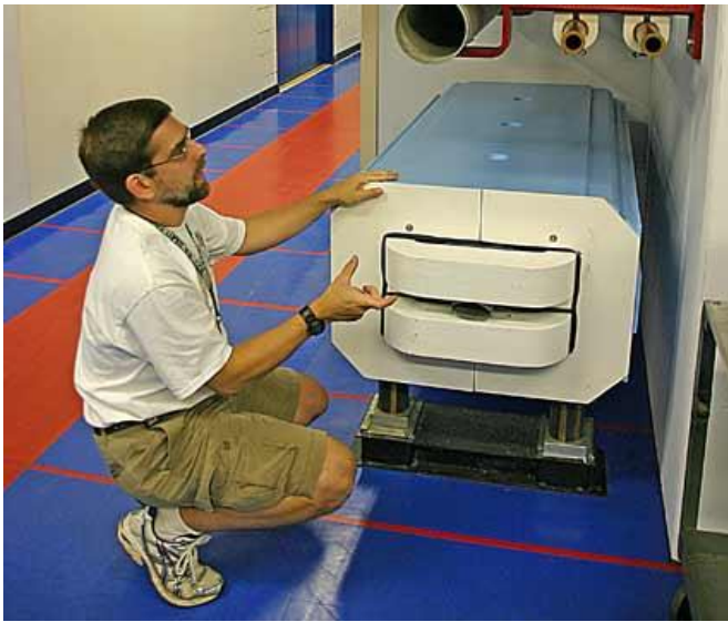
dipole bending magnet
