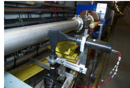
Plastic scintillator, \sim 10 \times 10 \times 1 \text{cm}^3
