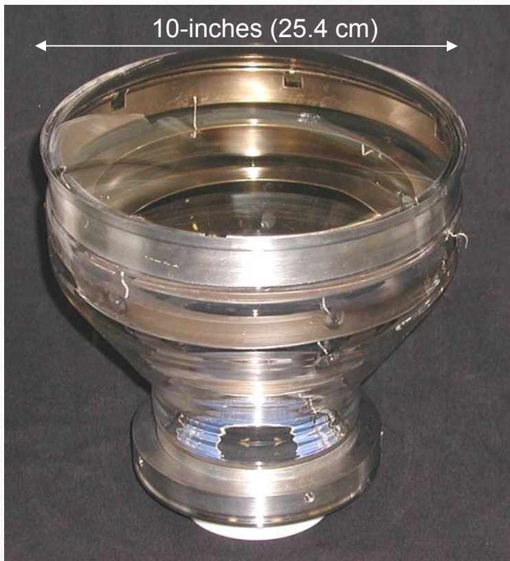
10-inch prototype HPD (CERN) for Air Shower Telescope CLUE.
