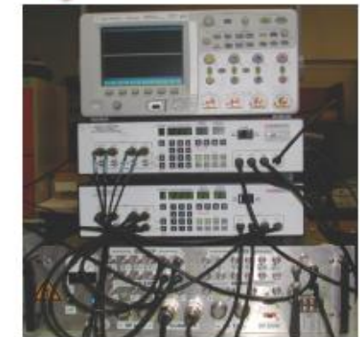
Amplifiers, filters input/output board for signal conditioning
