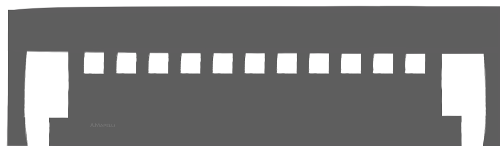
Plasma etching of fluidic openings
