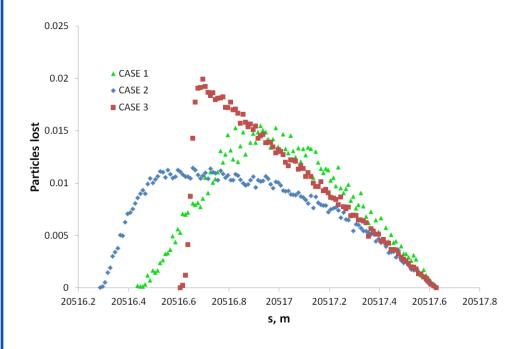
\* Results of the "old-concept" simulations: Matching of the tune was done after the orbital bump was applied
