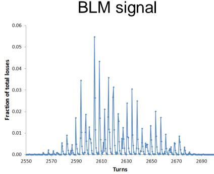
Combination of larger beam size and smaller offset provides better description of the time distribution Qx = 64.28, Qy = 57.31
