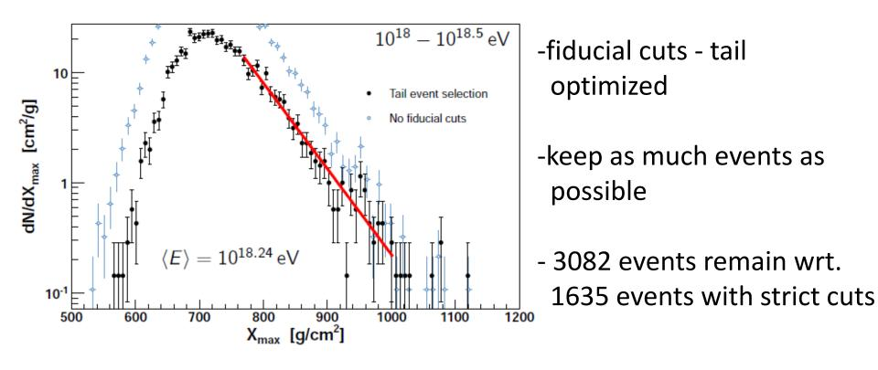
$\Lambda_{\eta}$  / g cm<sup>-2</sup> = 55.8 ± 2.3<sub>stat</sub> ± 1.6<sub>sys</sub> @ 10<sup>18.24 ± 0.005<sub>stat</sub> eV => Vs = 57 ± 0.3 TeV</sup>
