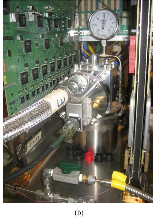
Figure 57: The Tracker Cryocooler cold head. a) Shows a schematic of the device, and b) shows the top half of the cryocooler, extending out of the cryostat body.
