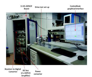
Rapid control prototyping of mathematical model (Simulink)
