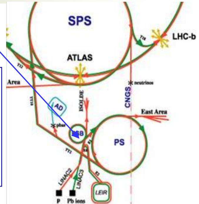
☞ *Incoherent tune shift* at injection  $\Delta Q \propto I/\beta\gamma^2 \rightarrow$  keep same tune shift with twice the intensity, increasing  $\beta\gamma^2$  by factor 2  $\rightarrow$  injection energy from 50 to **160 MeV**.
