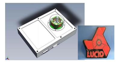
Langton Ultimate Cosmic ray Intensity Detector uses 5 Timepix chips to monitor the radiation environment in Space
