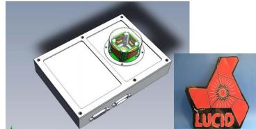
Langton Ultimate Cosmic ray Intensity Detector uses 5 Timepix chips to monitor the radiation environment in Space
