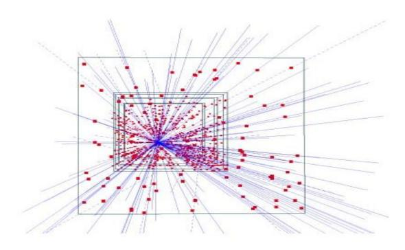
153 high energy particle tracks flying through a telescope of half a million pixels in the WA97 experiment back in 1995
