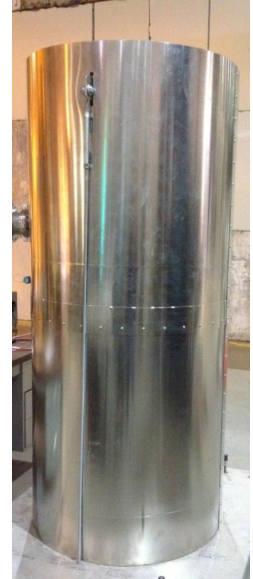
28" diameter vertical cryostat
