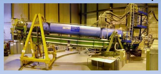
**The CERN Axion Solar Telescope (CAST)** aims to shed light on a 30 year old riddle of particle physics by detecting axions originating from the 15 million degree plasma in the Sun's core.
