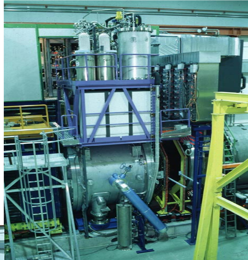
NA62: Liquid Krypton calorimeter(10'000 liters)
