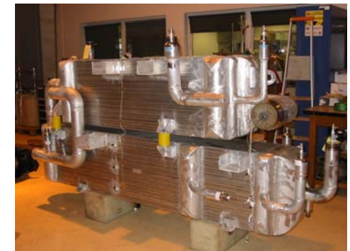
Heat exchangers before installation
