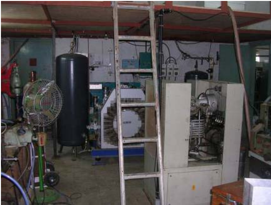
BAUER Model: G 150, 30 m 3 /hr; motor:11 KW
