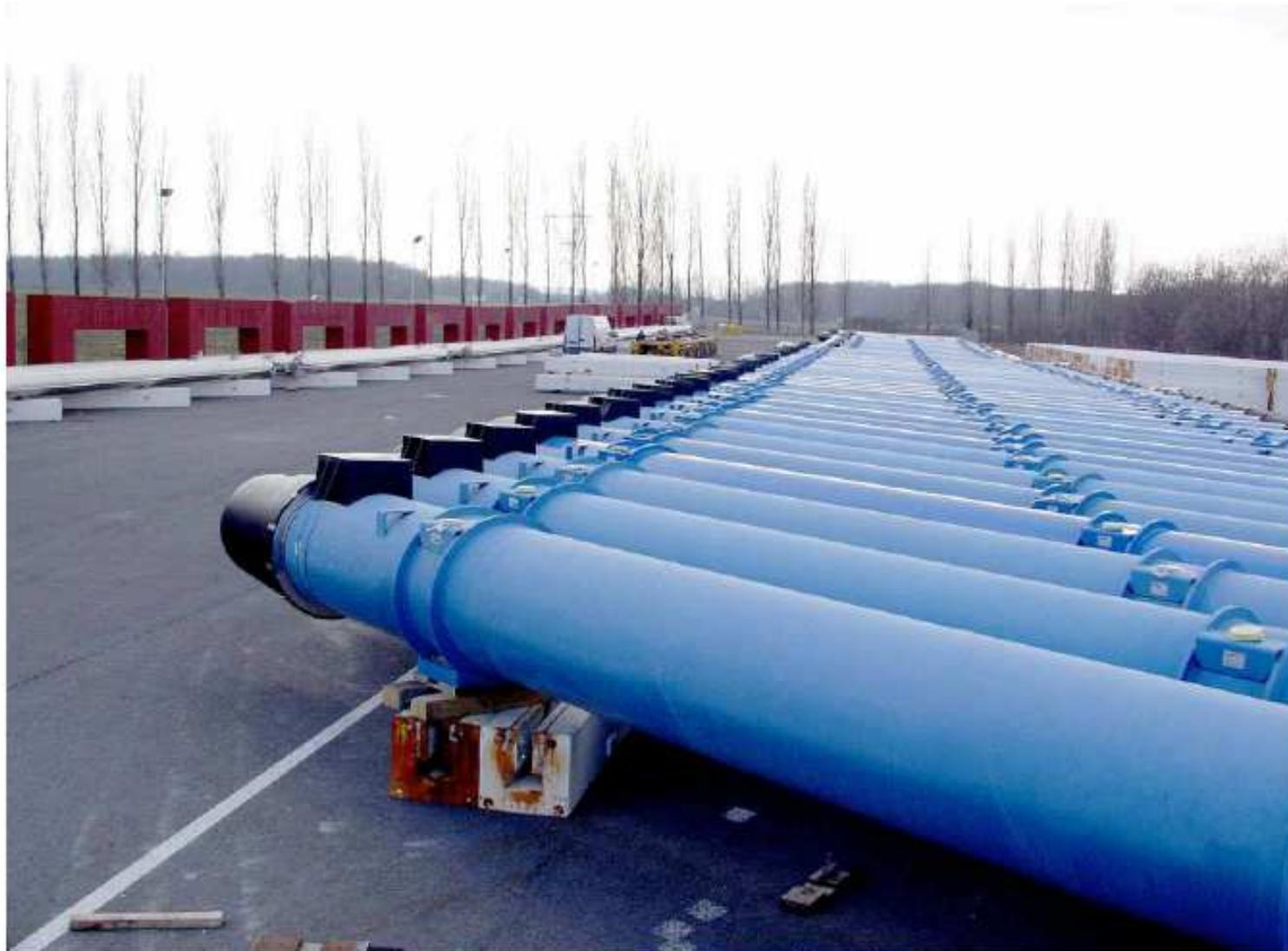
1232 superconducting magnets (before installation)
