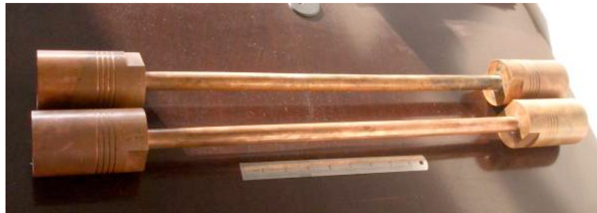
650A power leads
