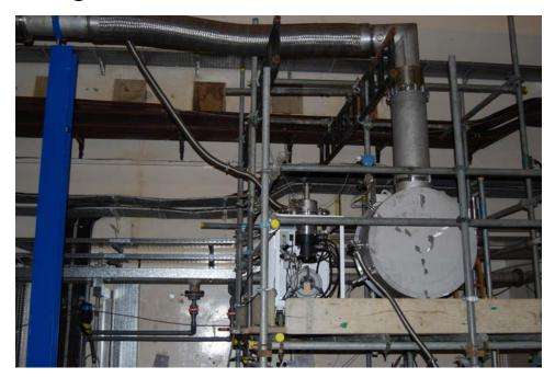
•34.5W guaranteed cooling power + 21.4W for current leads = 55.9W total + 10W for transfer line = 66W overall. This means that the test cap (plus transfer line) should be able to hold 56W – getting about 46W
