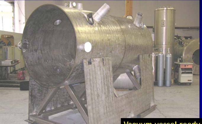
Vacuum vessel ready for assembly with cold mass
