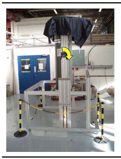
Tracker 1 is at present sitting in R8 at the Rutherford Lab. It is in the cosmic ray support frame in the vertical position. The frame was designed to allow the tracker to be installed in the horizontal position and then to be rotated to the position shown to optimise cosmic ray numbers. A value added to this is that we can use the same frame rotated to the horizontal to install the tracker into the beam line prior to the solenoids arriving should this be needed.
