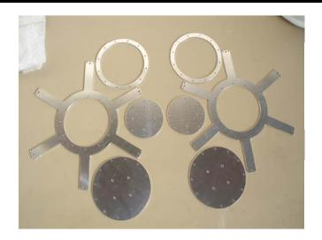
The fibre support masts are ready to be assembled. They consist of the aluminium components on the left. They are fitted with lengths of carbon fibre tubes. There is a rubber membrane at position 'x' to stop any off axis movement of the mast during installation being transferred as stress into the tracker.
