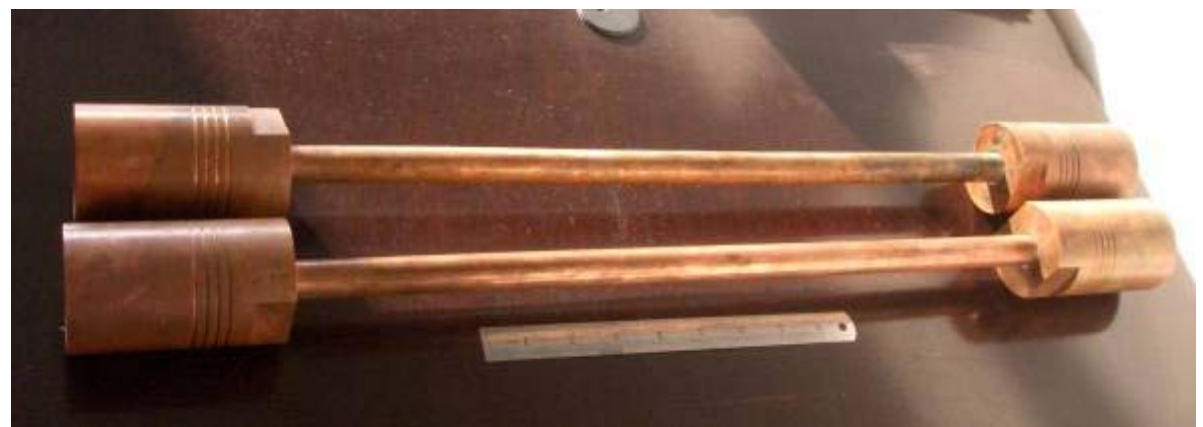
650A power leads
