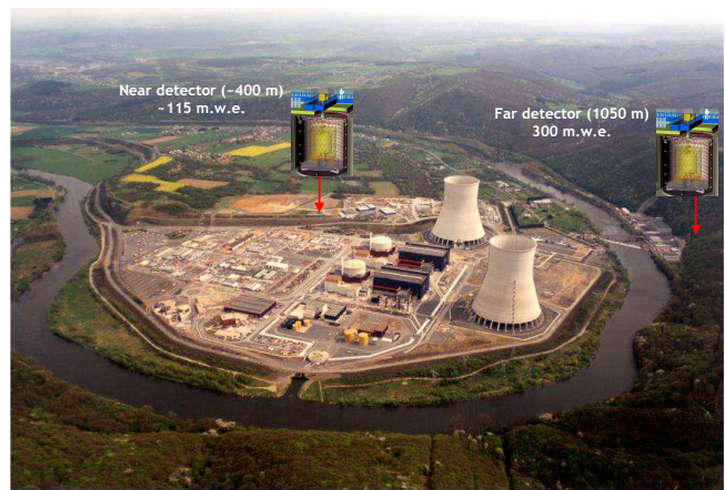
FIG. 1: Location of the two Double Chooz detectors in the Chooz-B nuclear power plant.
