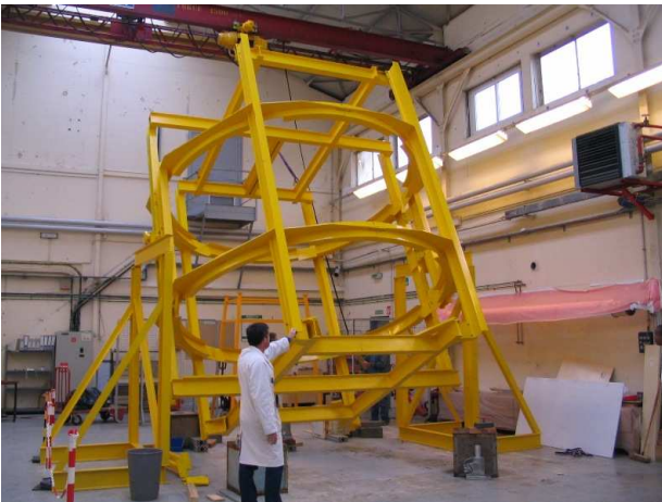
FIG. 5: Mechanical tool for the construction, transportation and installation of the \gamma -catcher vessel in the Chooz pit.
