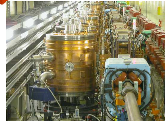
ARES RF cavities with higher energy storage ratio
