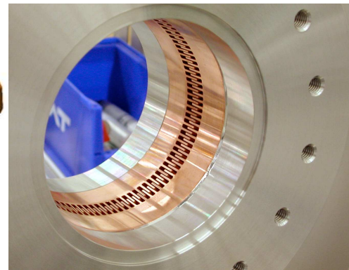
Antechamber beampipes and higher-current-proof bellows
