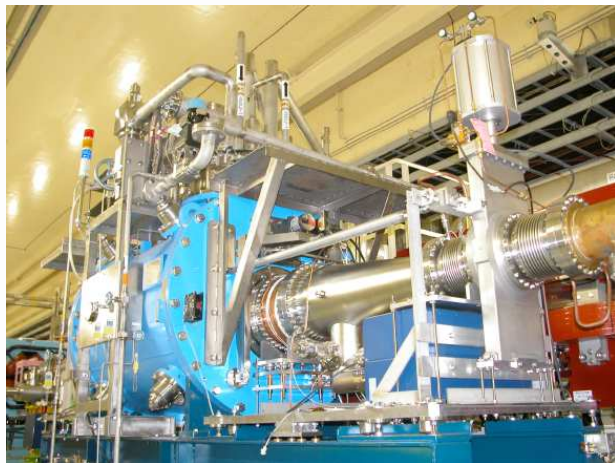
Superconducting cavities to absorb more HOM power up to 50 kW
