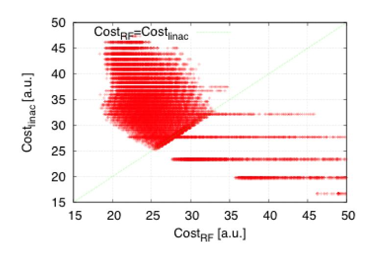
Higher Cost<sub>RF</sub>: Lower limit on G from beam dynamics Higher Cost<sub>linac</sub>: Upper limit on G from RF constraints
