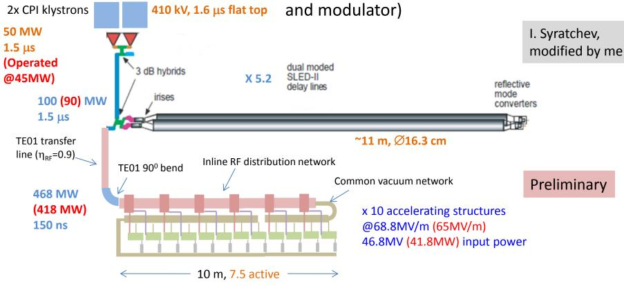
This unit should provide ~516 (488) MeV acceleration beam loading. Need 12 (12) RF units.
