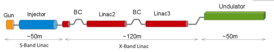
Looked a bit into a linac design for a typical Angstrøm FEL
