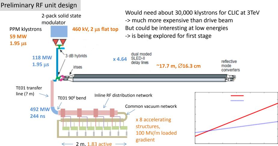
Compared to NLC, the energy gain per unit in CLIC'k case is 26% lower (need more klystrons per meter), but the unit length is ~ 3 time shorter.
