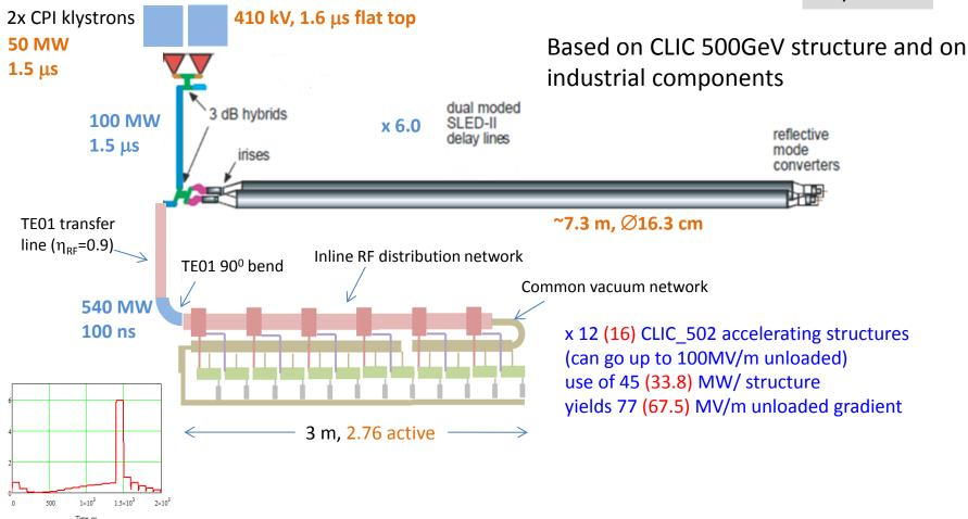
This unit should provide ~213 (248) MeV acceleration beam loading. Need 27 (23) RF units.
