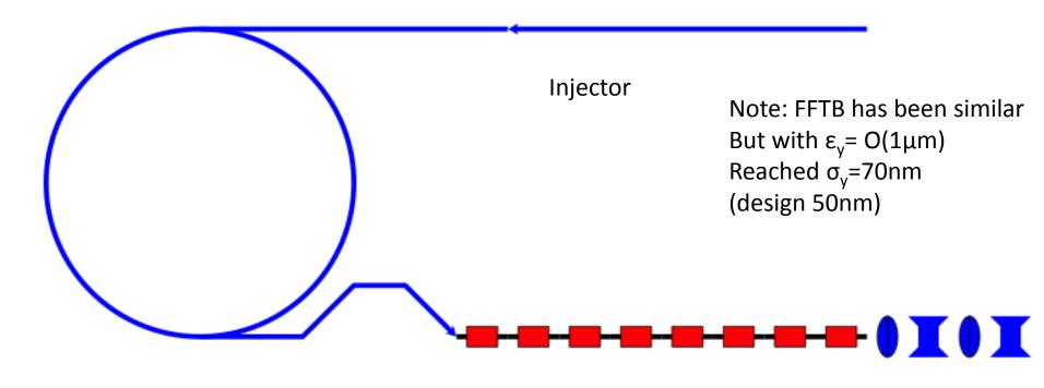
Low emittance ring, e.g. CLIC damping ring, 3<sup>rd</sup> generation light source, damping ring test facility
