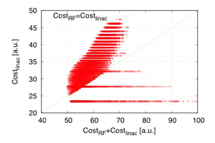
Lowest cost machine has slightly larger linac cost compared to RF cost
