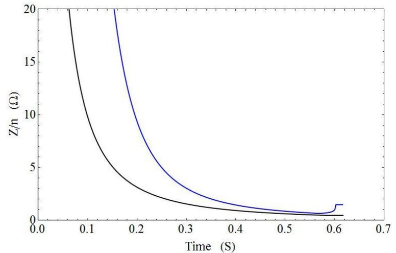
After calculation the longitudinal emittance must be increased up to 1 eV.s in order to maintain Threshold value above space charge impedance.
