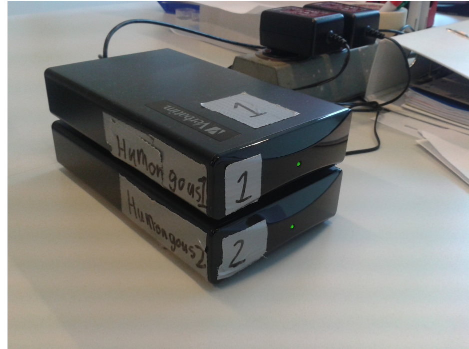
Harddrives “humongous1” and “humongous2” (2x 2 TB) for local scratch space (USB drives are cheap, local, and unbureaucratic..)
