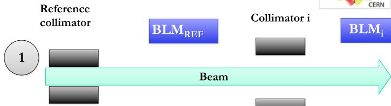
2. The collimator i is aligned to the beam.
