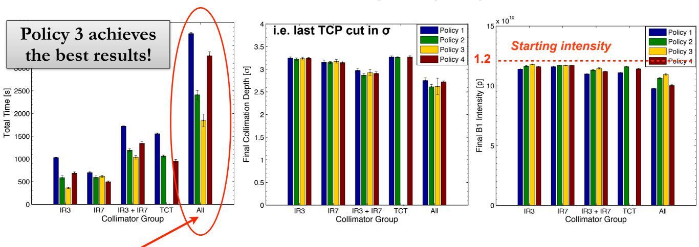
• Policy 4: gain in time is larger when all collimators are moved simultaneously (Policy 3), even though there are more frequent interruptions.
