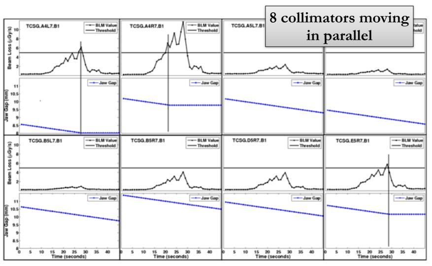
• Iterative algorithm to determine which collimator is at the beam after BLM signal crosstalk.
