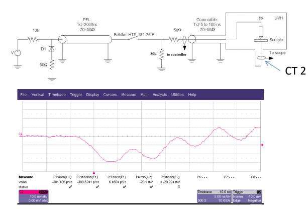
In this position the current transformer is insensitive to as much stray capacitance as possible
