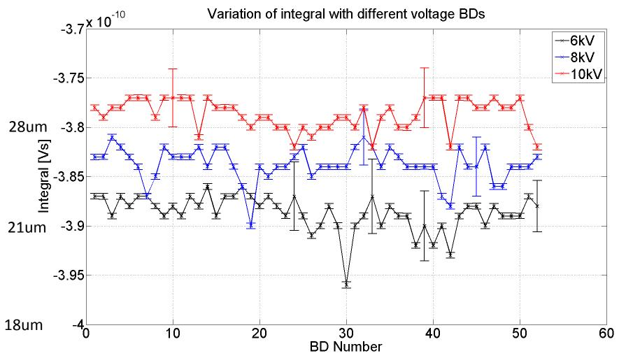
Hypothesis that gap would change more with higher voltage  $\rightarrow$  more damage to electrodes not proven. Sorry for lack of proper um scale.
