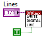
Figure 2 Switch control with "write_dig_line_DigitalOutput.vi" with NI-DAQmx.
